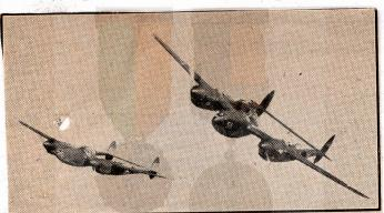
'his flying view of Lockheed P-38 "Lightnings" shows well the wide tail unit and he dihedral of the wings. (See special article on page 5). Photograph by courtesy of the Lockheed Aircraft Corporation, U.S.A.
